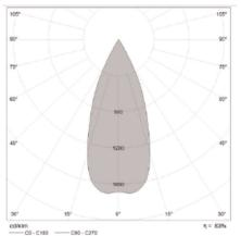
Correlated color temperature: 3000 – 6000 kelvin Rated median useful life: 50000h L70 at 25°C Luminaire input power: 3 w
